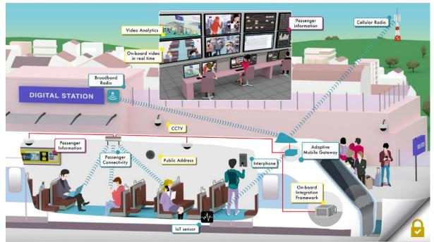
©Thales - All onboard services are connected to the Operation Control Centre (OCC) via secure communications
